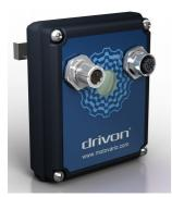
This optional module implements hardware and software interfaces for Real-Time-Ethernet networks over Ethercat profile. Two M12 D-code connectors (a male and a female connector) are provided on the outside of the module for Line connection to field network.
